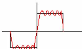
The behavior of a Fourier series near a discontinuous point of  $f(x)$  is known as Gibb Phenomenon.
