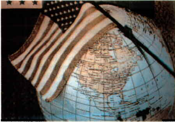
FIGURE 2. PHOTOGRAPH OF RECONSTRUCTED COLOR IMAGE USING BLUE-GREEN FILTER OVER THE SHORT WAVELENGTH RECORD. NOTE THAT THE ORIGINAL SCENE CONTAINED YELLOW AND GREEN IN BACKGROUND.
