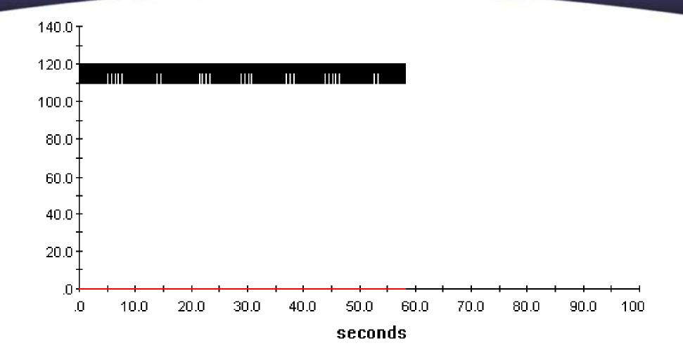
No packet loss shown at 1% load
