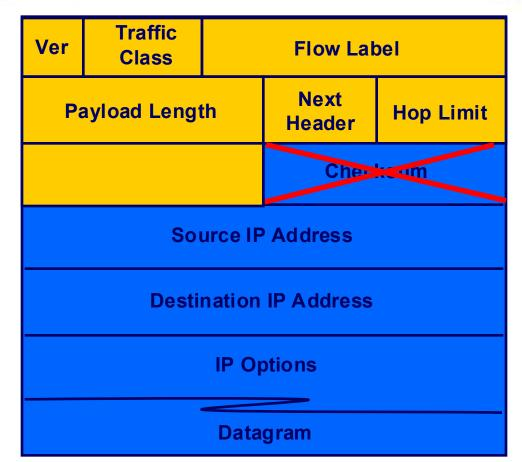
Since upper layer protocols like TCP and UDP calculate their own checksums, the IP header checksum was considered unnecessary. If content authentication is desired, the Authentication header is available in IPv6.
