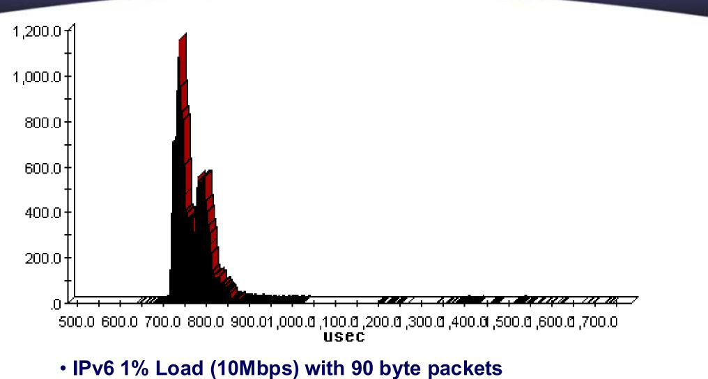
Notice IPv6 latency three times that of IPv4
