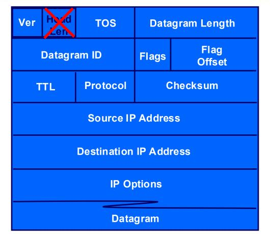
IPv4s "options" necessitated the Header Length field, as headers could be anywhere from 20 to 60 bytes. Now there is no need.
