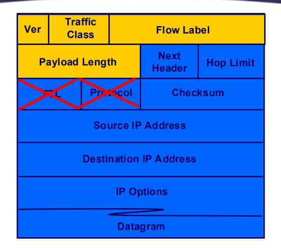
The "Next Header" field can indicate which type of extension header follows the IPv6 header. This overcomes the need for the IPv4 "Protocol" field. TTL is replaced by "Hop Limit."
