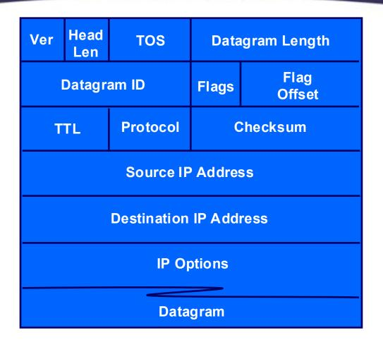
Here is the traditional IPv4 Header. Watch the IPv6 Transformation!
