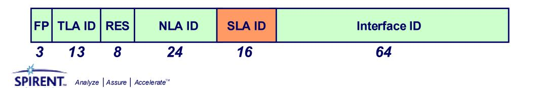
V6 host addresses are recommended (not mandated!) to be built from so-called EUI64 addresses. EUI64 addresses are -- as the name says -- 64-bits wide, and derived from MAC addresses of the underlying network interface. For example, with Ethernet, the 6byte (48-bit) MAC address is filled with the hex bits "fffe" in the middle -- the MAC address
