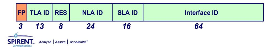
The Top Level Aggregation IDentifier contains the highest level routing information for the address. This space will typically be assigned to transit providers, not leaf sites. At 13 bits, this assures that there can only be 8192 different top-level routes in the internet.
