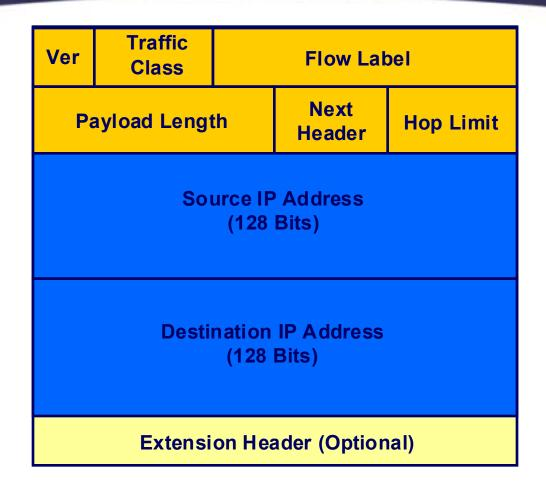
Finally, the main reason for IPv6's existence is the 128 bit addressing scheme. Extension headers are available for a number of different functions, but are not considered part of the IPv6 header itself.
