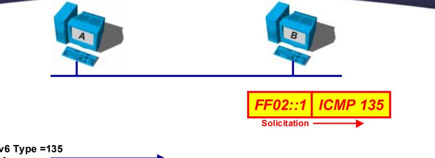
ICMPv6 Type =135 Src = A Dst = Solicited-node multicast of B Data =Link layer address of A Query = what is your link address?
